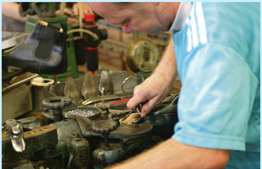
Figure 3: Toe lasting with a bed lasting machine
