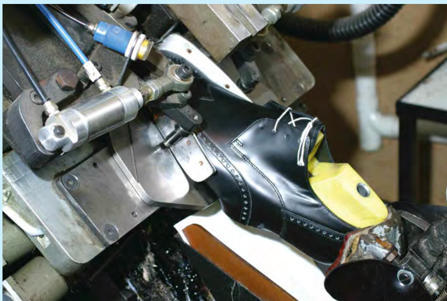
Figure 4: Automatic toe lasting increases production
