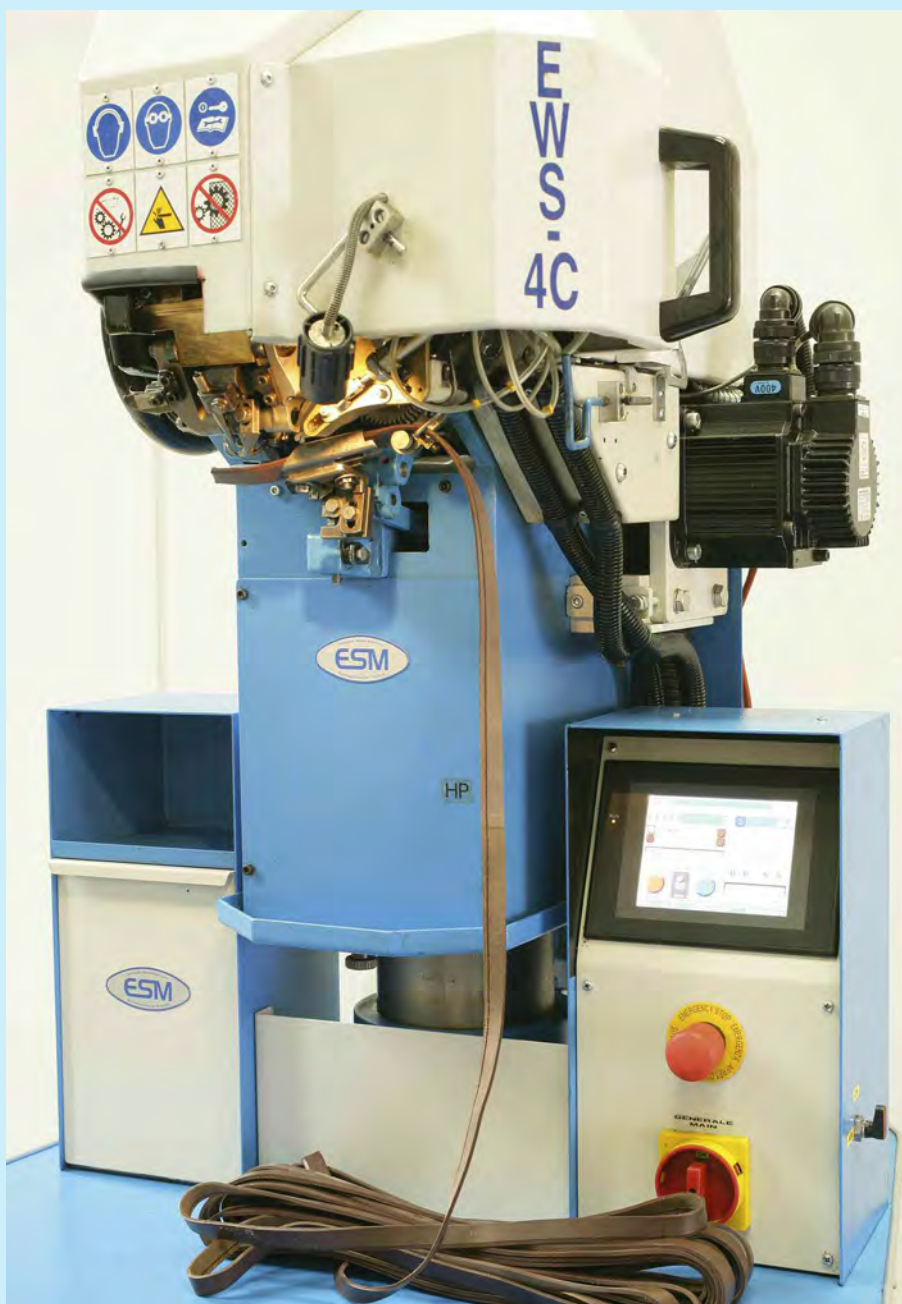
Figure 7: Recently-developed walt sewing machine with touch screen interface
