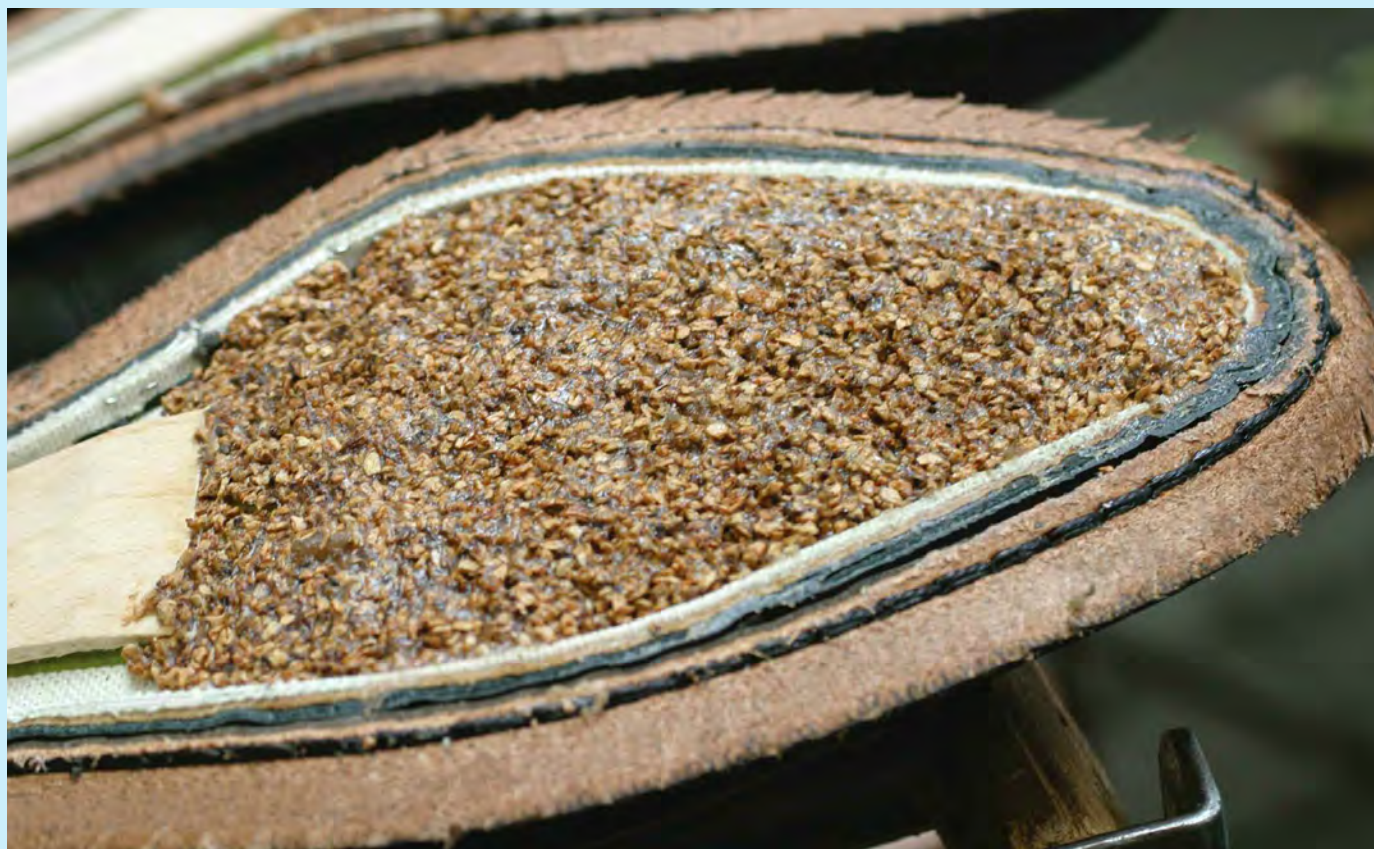
Figure 9: Cork bottom filler aids comfort and insulation
