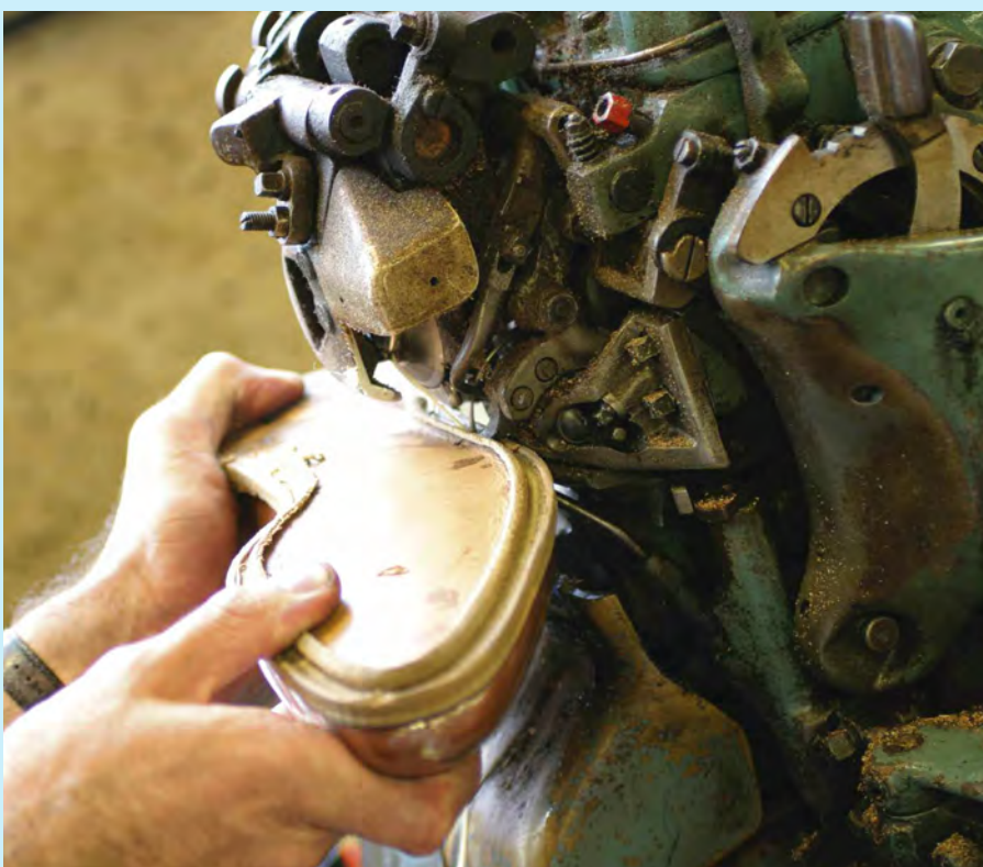
Figure 11: Channelled sole attached using a lockstitch
