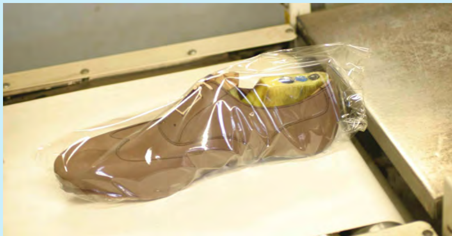
Figure 6: Shrink wrapping minimises damage to the upper
