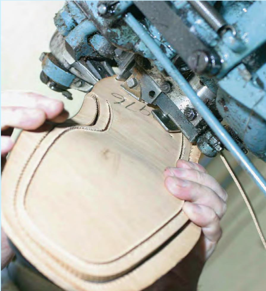
Figure 10: Rounding down the sole and groove cutting
